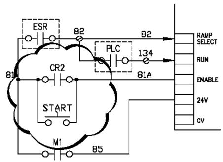
**This change is at the VFD**. Wire 81 goes to CR2, NO contact and a new momentary contact in the key switch, actuated when the key switch is in the START position. New wire 81A is wired in parallel with the output of these two contacts. Wire 81A terminates on the AC VFD where 81 was formerly terminated.
