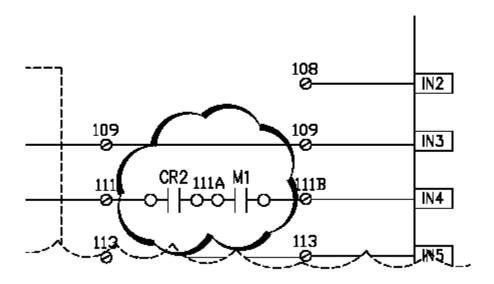
Wiring change at the PLC. Input 4 of the PLC, wire #111, is to be removed and connected to CR2, NO contact. A new wire is to be installed to this NO contact, wire #111A and run to M1, NO contact. From this contact block a new wire #111B is to be installed in the PLC at input 4, formerly where wire #111 was terminated.
