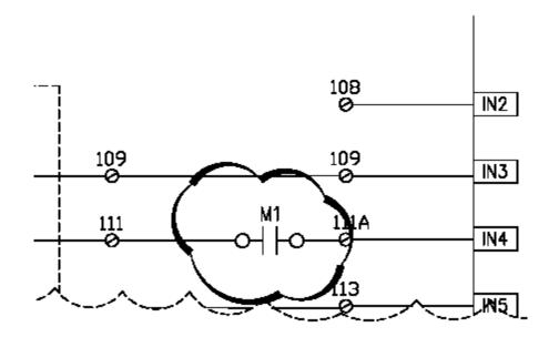
**This change is at the PLC.** Input 4 of the PLC, wire #111, is to be removed and connected to M1, NO contact. A new wire is to be installed to this NO contact, wire #111A and installed in the PLC at input 4, formerly where wire #111 was terminated.
