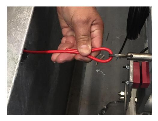
The cable wire or lanyard goes through the 90-degree elbow to the outside.
