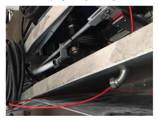
And then run it up a control post and just have a quick release at the end of the conveyor with a pull cord and T-Handle, like a lawn mower pull cord. We currently have this quick release pull kit ready to be ordered.
